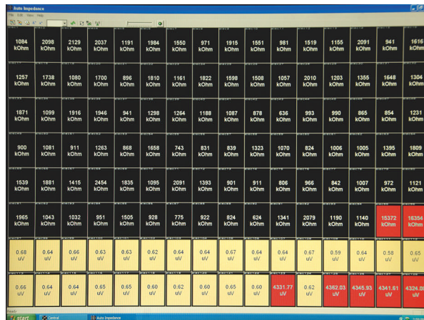
With the automated impedance tester, operators can quickly identify which electrodes are operating within specific ranges, such as between 200 and 400 kΩ. The channels within that range will show up as black, those above the range in red, and those below the range in yellow.
