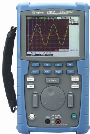
Agilent's U1604A provides both a wheel and buttons for setting the instrument.
