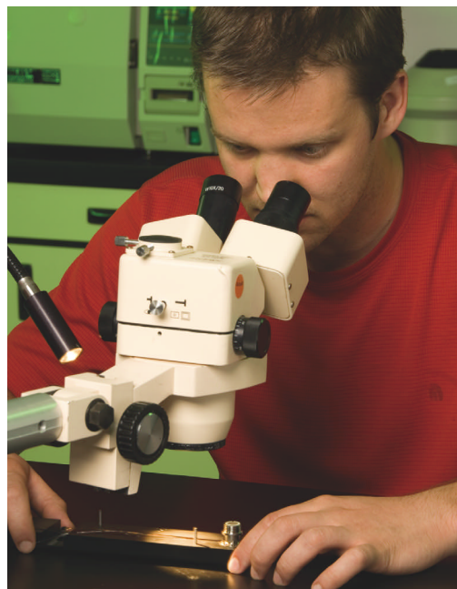
Engineer Rick Van Wagenen does a microscopic inspection of BrainGate’s electrode leads, one of a long litany of procedures performed on the system.
